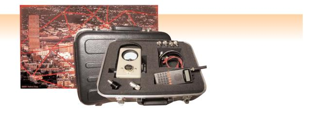
To facilitate efficient installation of a Keltron wireless network, Keltron offers an installation kit with all the equipment necessary to prepare, install and test the network.
